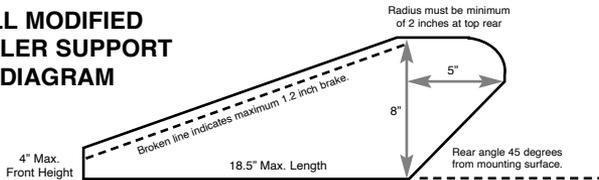
No more than 3 spoiler supports permitted (a 1" steel strap is not considered a spoiler brace). Front edge of spoiler support must be inline.
