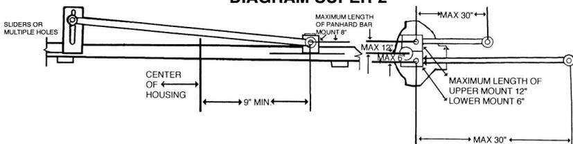
the rearend. No anti-sway bar may be used on the rear. No lift bars, snubber bars, J-bars or any other traction devices allowed. Panhard bar allowed on 3-link suspension only.
